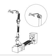
Step 5: Using the 5 mm Allen Wrench loosen the handlebar clamp.
