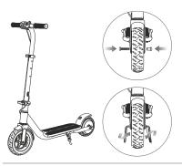
Step 8: Put the tire to the right place, tightening the screw. Use the Allen Wrench to tightening the screw.
