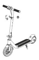
To adjust the height of the handlebars, open the quick-release lever and slide the T-bar to the desired position and resecure the quick-release lever to lock into place.
