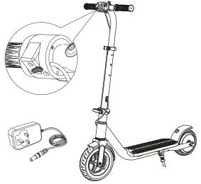
Plug the charger plug into wall outlet, the light on the charger should be green.
