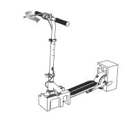
Step 7: Using the 5mm Allen Wrench tighten the hanclebar clamp.
