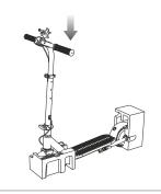
Step 6: Insert the handlebar with the throttle facing the rider.
